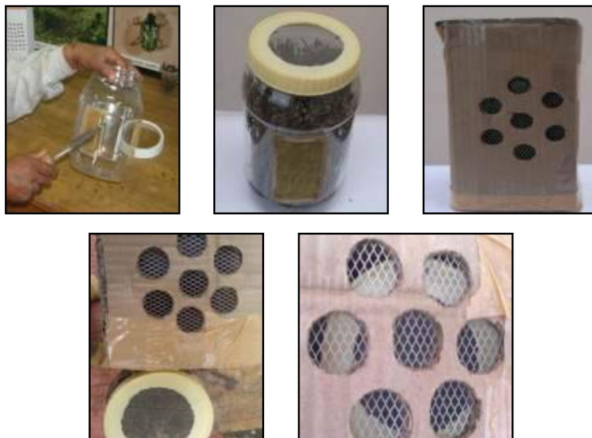
Fitting of brass or soft iron wire mesh windows on side walls of the container and on the lid of the plastic containers with the help of soldering unit. The side and top view of cardboard box with iron wire mesh to prevent the damage to container kept inside with bioagent
