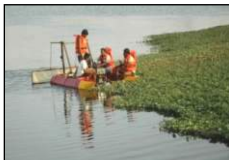
Engine powered aquatic weed cutter in operation
