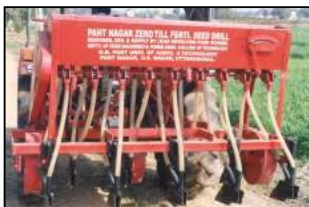
Zero-till seed-cum-fertilizer drill with knife-type tynes for sowing of wheat
