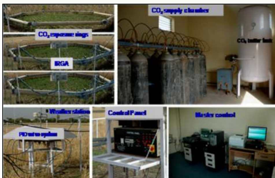
Different components of Free Air CO 2 Enrichment (FACE) facility
