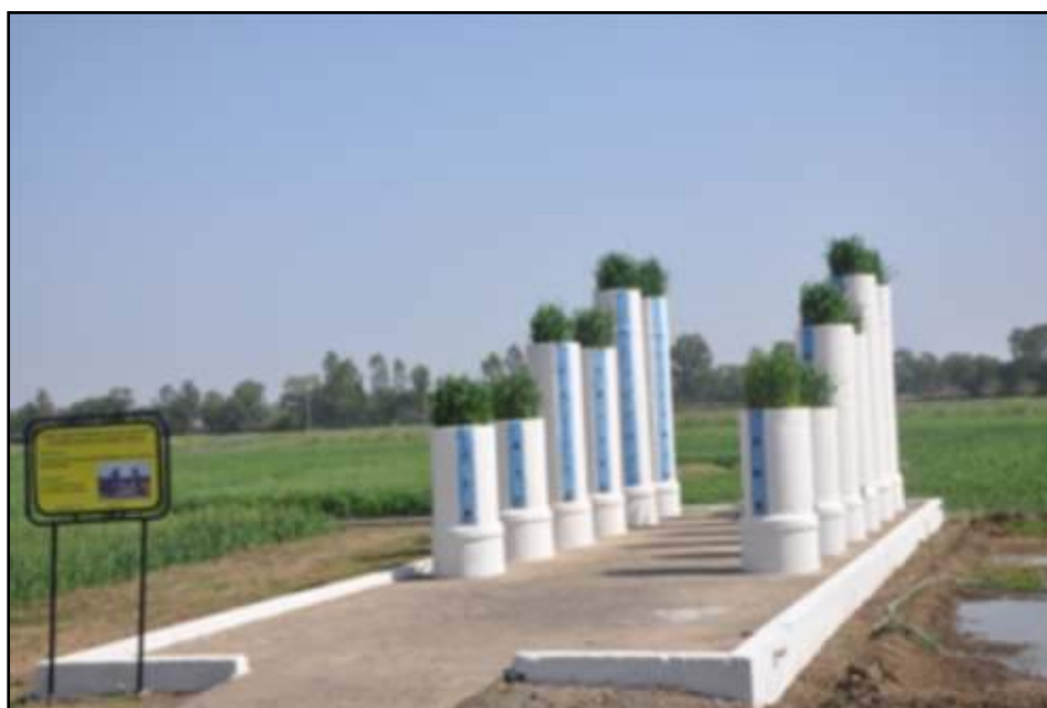
An overview of field lysimeter having provision for collection of soil samples and leachates.
