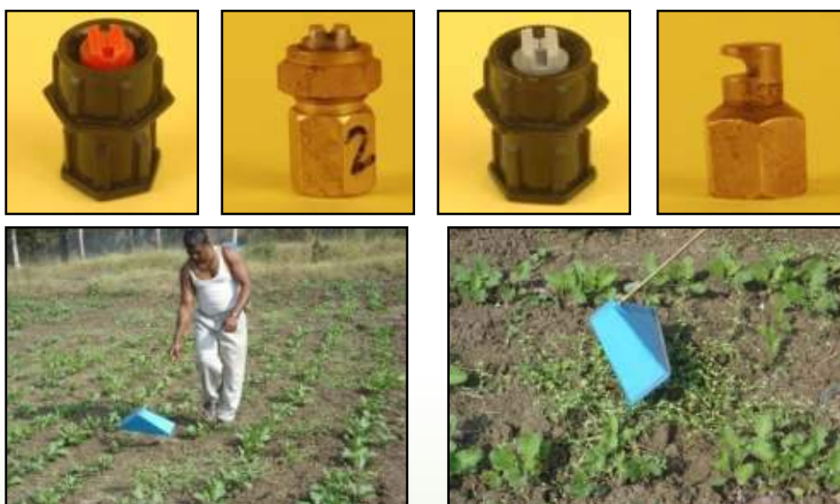
Spraying of herbicide using Fan Nozzle with plastic hood.
