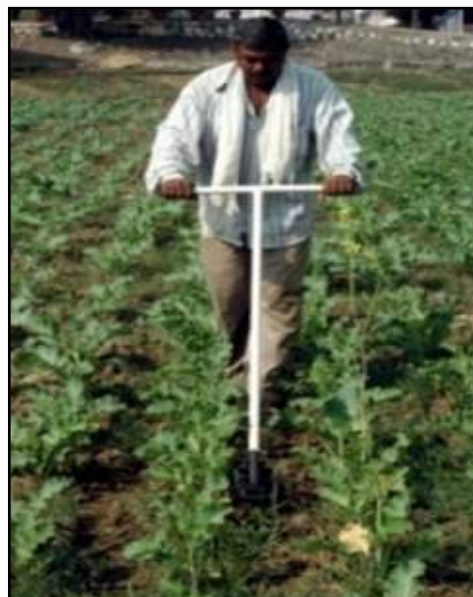
Twin wheel hoe weeder in operation
