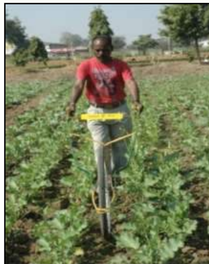
Cycle wheel-hoe weeder in operation
