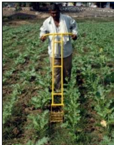
Rotary push type weeder in operation
